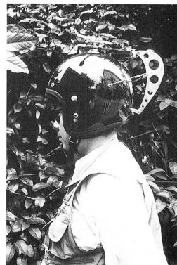
Helmet This helmet can switch the direction from which auditory stimuli are heard, from right to left.
